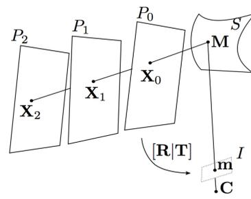
The relative poses of the reference plane under three distinct poses can be estimated using reflection correspondences established across the images<sup>1</sup>. We can then form a 3D Plücker line  $\mathcal{L}$  from the reflection correspondences of each observed point  $x$  in the image.
